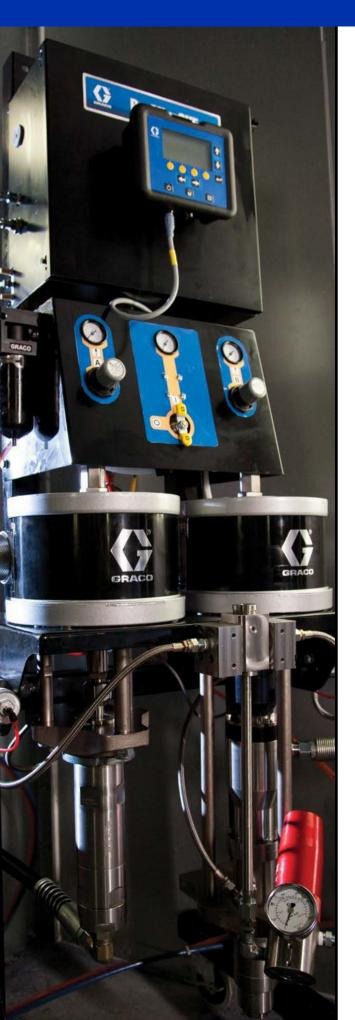
Intuitive, icon-driven LCD display allows you to set up, operate and monitor the system as it performs.
